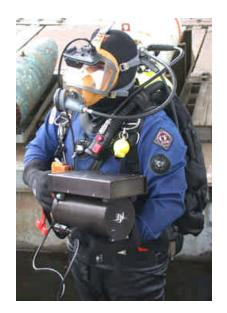
Fig. 6. A handle and head-mounted display were added to the DIDSON for this exercise. A cable connected the sonar to topside for commands and data transfer. A monocular version of the display is on the diver's mask.
