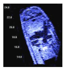
Fig. 8. A DIDSON image of the stern of vessel resting in 10 m of water. This image was taken in the low-resolution mode. The range scale is in meters.
