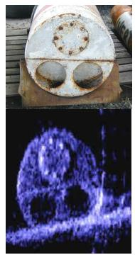
Fig. 10. Photograph and a DIDSON image of a mine shape.
