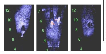
Fig. 5. Three sample images taken with the LIMIS. The left image shows a limpet mine on the hull of a ship 7 feet (2.1 m) from the sonar. The center image shows two hands. The right image shows an intake on the hull of a ship. The intake is approximately 46 cm in diameter and is 9 feet (2.7 m) from the sonar. The left and right images were taken in Chesapeake Bay in water with 15-cm visibility.
