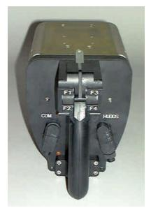
Fig. 2. Five thumb switches control the LIMIS. The four labeled F1-F4 control software commands. The fifth, between F1 and F3 controls focus. The COM port is an RS-232 link to download commands that duplicate F1-F4 controls and to upload stored digital images. The HUDDS port connects to the mask-mounted display.
