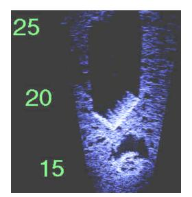
Fig. 4. A LIMIS image of a 50-gallon drum at 20 feet and an old tire at 15 feet.
