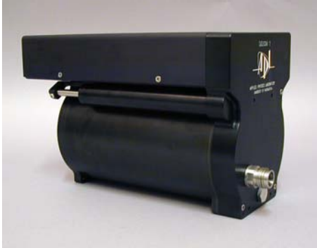
Fig. 1. Side view of DIDSON. The lenses are in the upper rectangular compartment. The electronics are in the cylindrical housing. A focus motor moves the center lens element fore and aft to focus on objects from 1 m to max range.
