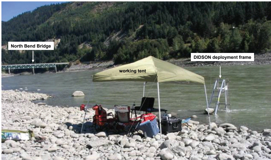
Figure 34. Photo showing the DIDSON deployment site at Boston Bar. Also shown is the working tent on the right bank for shielding electronics and computer equipment used for data collection.
